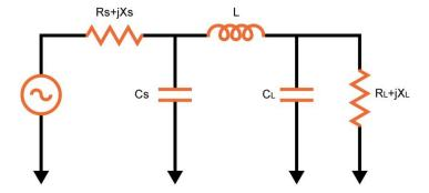
The AC generator on the left represents the transmitter output circuit, with a typical output impedance of a few ohms, up to typically 50ohms.
