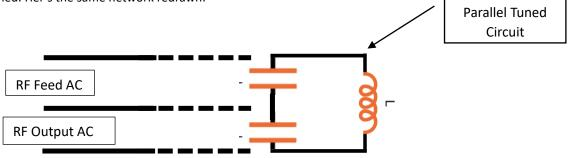
Now we have the same matching network, but re-arranged into a more familiar shape, that of a parallel tuned circuit, which is exactly what it is!
