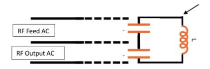
Now we have the same matching network, but re-arranged into a more familiar shape, that of a parallel tuned circuit, which is exactly what it is!
